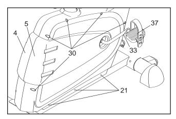
Shield. Using an adjustable wrench, turn the Right Pedal (37) counterclockwise and remove it. Next, turn the Crank (33) so that it points toward the front of the exercise cycle, and then slide off the Right Side Shield.
